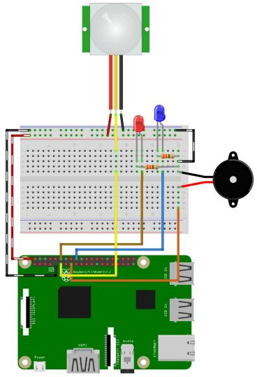
The Alarm circuit combines the PIR circuit and the LED/Buzzer circuit from Worksheet Two. You will be using this to create a simple movement alarm.
