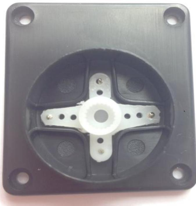
After finished above, sway the servo from side to side, let the servo face in the front in 90 degree. Install the copper column and fix up the middle screw.
