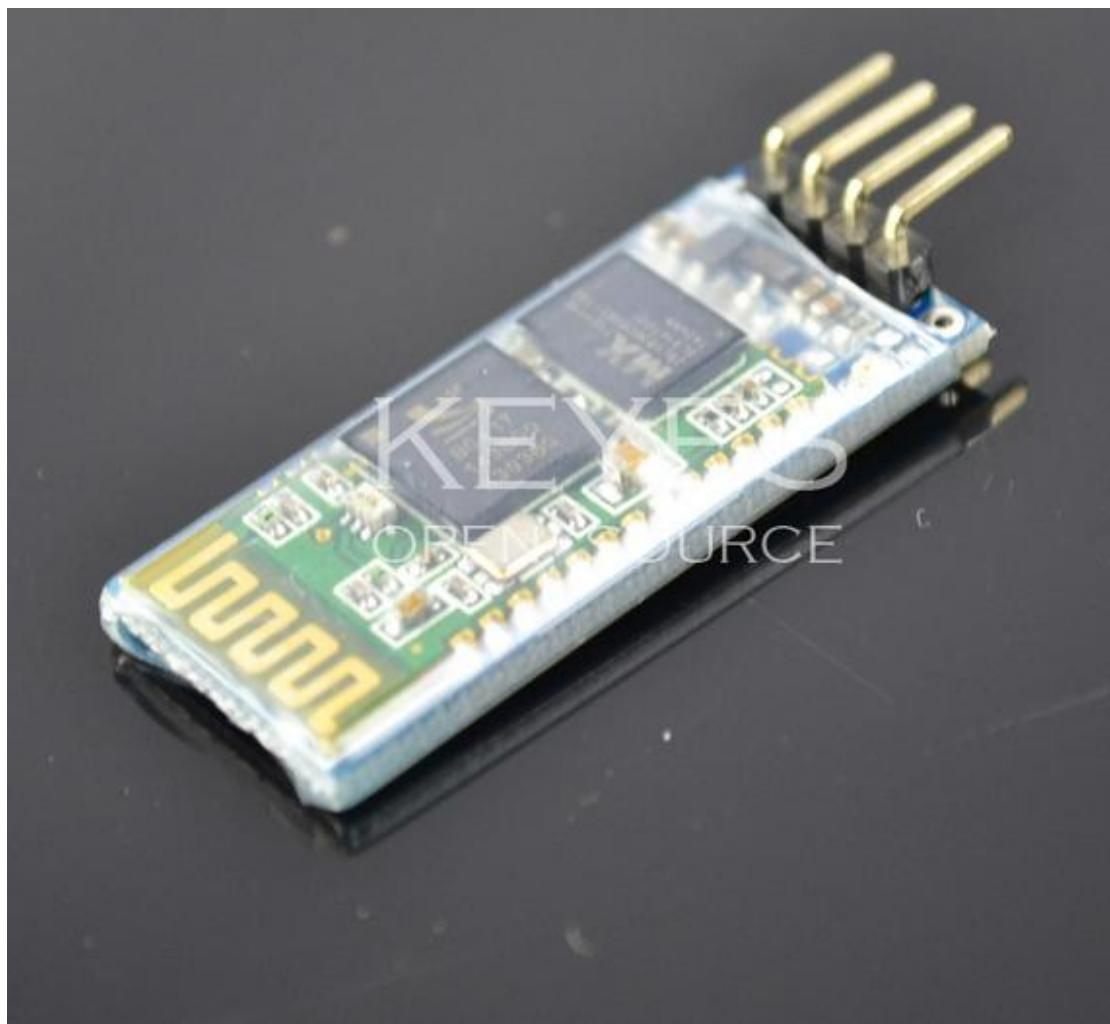
In fact, the Bluetooth serial port, have put Bluetooth serial process, install the drivers, we can regard it as a serial port to use. We talk about the PC machine driven how to install Bluetooth adapter, and connect to the Arduino.
